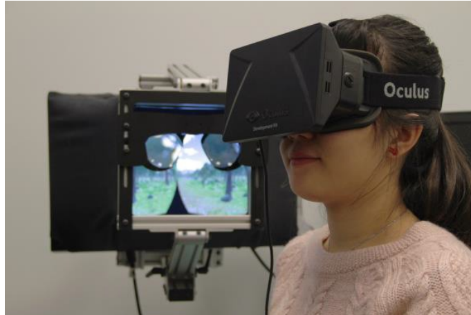
Figure 2. The current experiment setup with the user immersed in the VR environment through an Oculus Rift Head-mounted Display (the one on the model's head). To return focus to the physical environment (i.e., to “escape” the VR environment), the user must remove the HMD.
